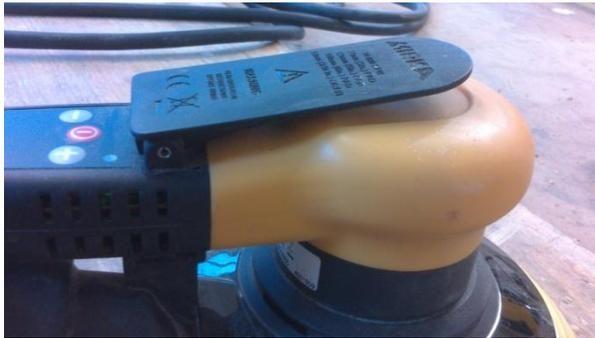
*Power on/off and speed adjuster buttons.*
