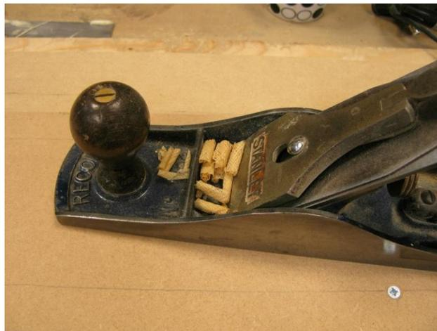
To true up veneer. Tap the veneer leaves down so the edges are aligned and lay them on the top board so they are protruding by about 2mm. Lay a board on top with a weight on top to compress the veneers (others use a clamping system, but I find this works OK). Run the plane along the veneer edge using only light pressure until the edges are smooth and true.
