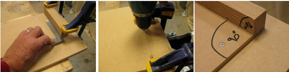
Screw a block to the underneath of the other end of the board, this is to act as a hook against the edge of the bench to aid stability in use.
