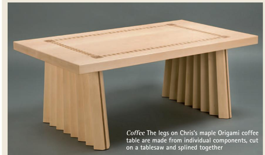
*Coffee* The legs on Chris's maple Origami coffee table are made from individual components, cut on a tablesaw and splined together
