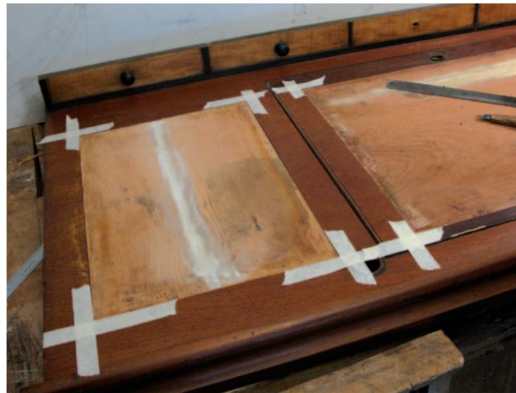
the leather surface will be flush with the surround. If the new leathers are thicker than the previous ones the surface may need a little chamfering to allow for the increased thickness. So that you don't damage the edge, perhaps even pulling it up when chamfering, use a scalpel and rule to score the grain up against the edge, then pare a 15mm-wide margin until the leather fits flush.
