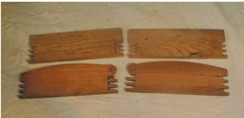
Box sides before shaping (top) and after shaping (bottom) – note over-length pins
