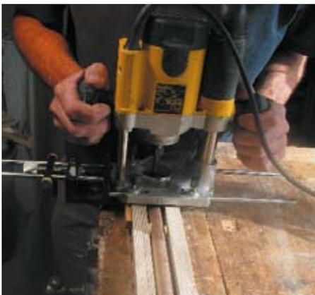
**Set-up for routing the groove**
