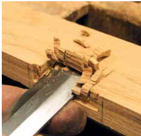
▲ Pic.17 ...methodically using a well-fettled chisel...
