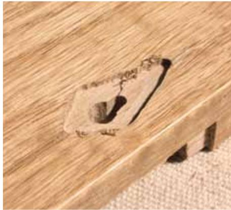
▲ Pic.35 Again, when routing out the diamond recess, Chris made his final cuts with a chisel...
