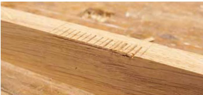
▲ Pic.7 ...but he could have used a chisel, chopping down across the grain to remove...
