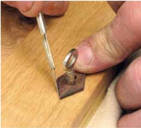
▲ Pic.34 The points of the escutcheon were aligned and marked
