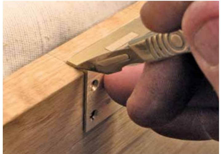
▲ Pic.22 ...using a scalpel to make the finest marks...
