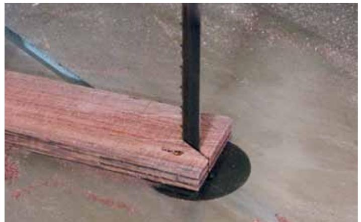
▲ Pic.33 ...then the diamond shapes were cut on the bandsaw
