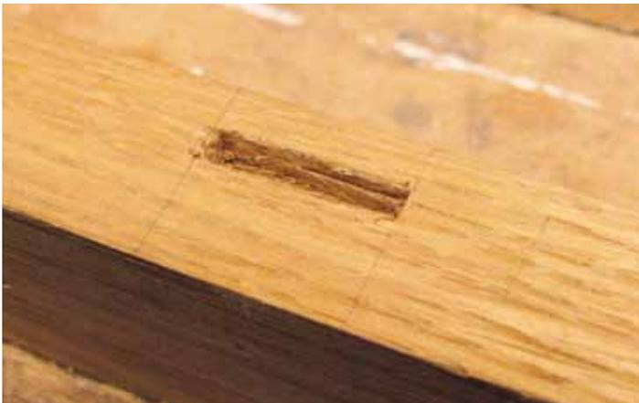
▲ Pic.40 ...then either routing or chopping out the slot
