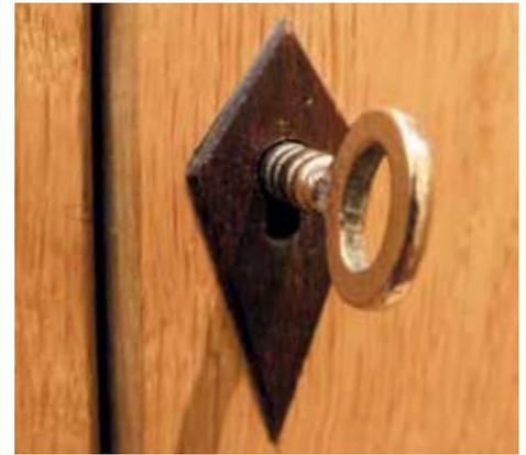
▲ Pic.36 ...before gluing the escutcheon into the recess
