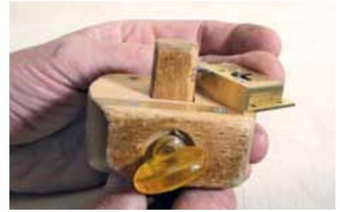
▲ Pic.4 After setting the marking gauge to the depth of the top plate...
