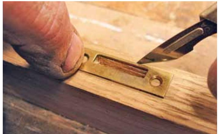
▲ Pic.41 The aligned cover plate was marked with a scalpel prior to its recess being cut
