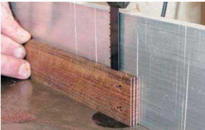
▲ Pic.32 Each layer was bandsawn to about 3mm thick...
