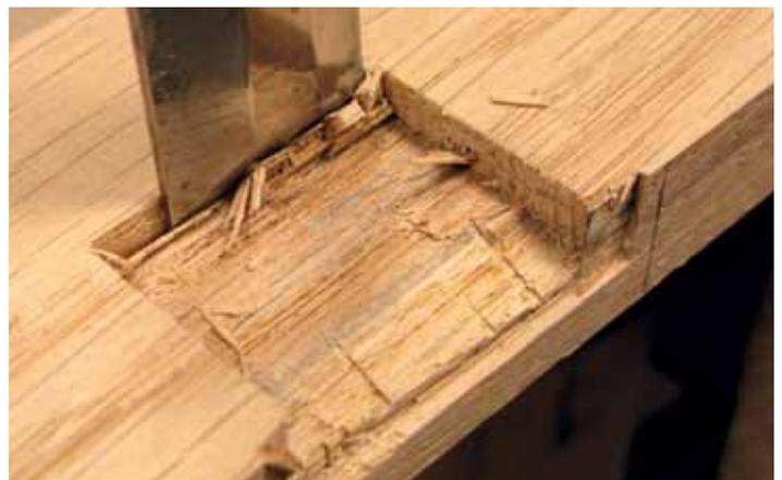
▲ Pic.20 ...that can be removed by cutting along the grain
