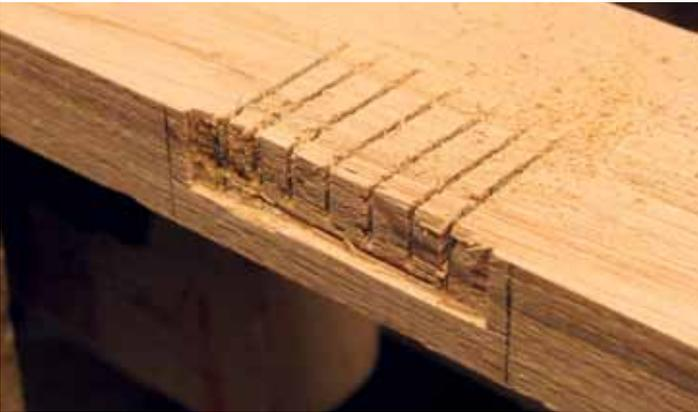
▲ Pic.14 ...or by making a series of angled saw cuts to break up the waste
