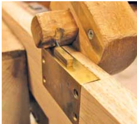
▲ Pic.38 ...setting the gauge to the bolt from the door front...
