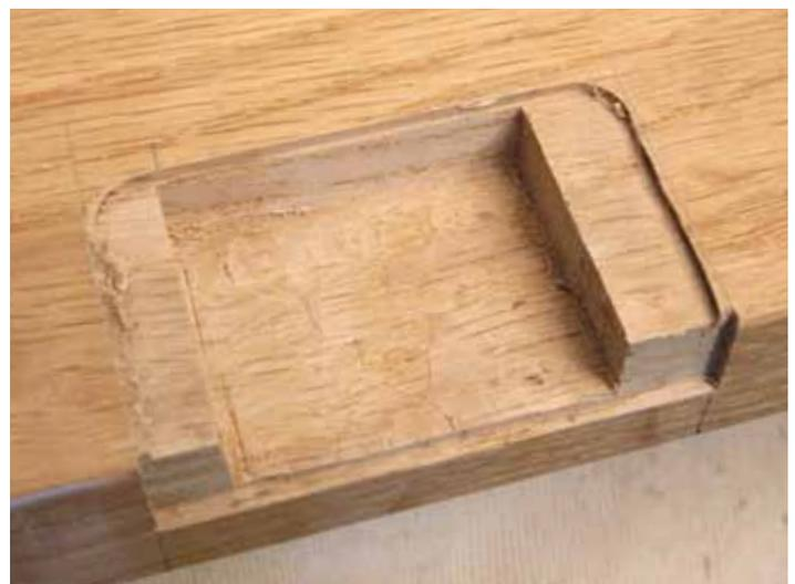
▲ Pic.25 ...but left the final detailed cuts for the chisel
