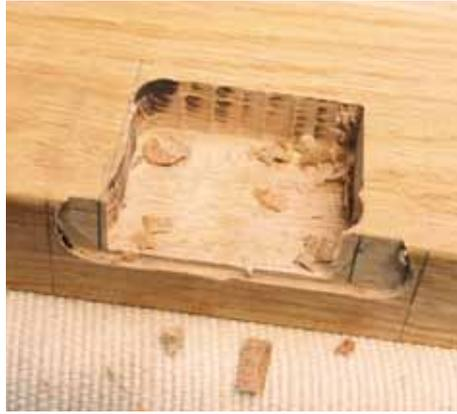
▲ Pic.12 ...recess depth to a tad more than the thickness of the body plus the back plate
