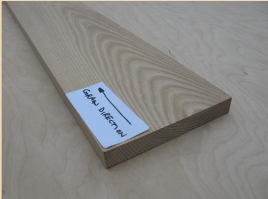
Annual rings curve up to the base of cathedral window. Plane from base upwards.
