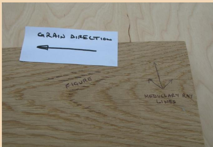
Face of oak board showing figure and grain directions.
