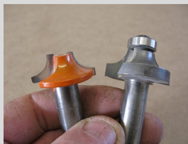
Ovolo moulding cutters, bearing guided on right.
