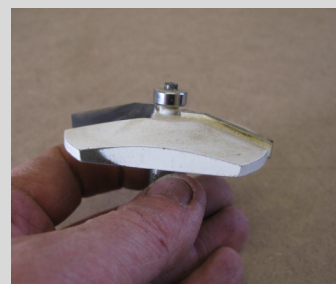
Fielding cutter, to be used only in router table.
