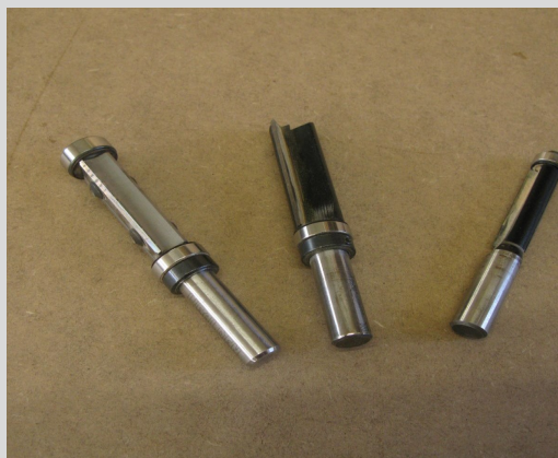
Bearing guided straight cutters, note different bearing positions.
