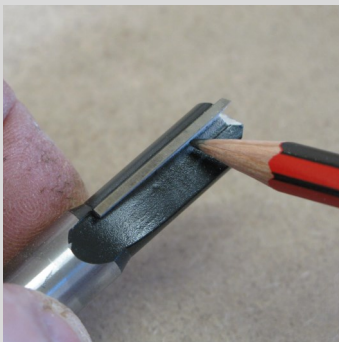
Straight flute cutter with Tungsten carbide tips.
