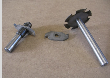
Grooving cutters with additional cutter in centre.
