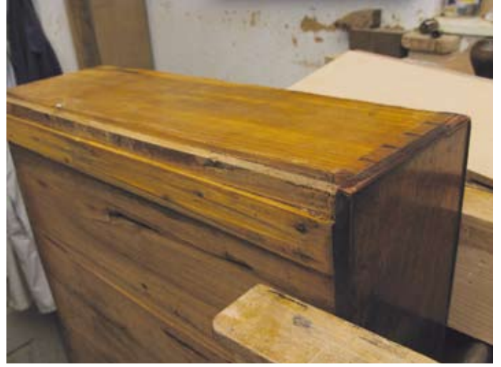
16 L-shaped area removed from bottom of badly damaged drawer side
