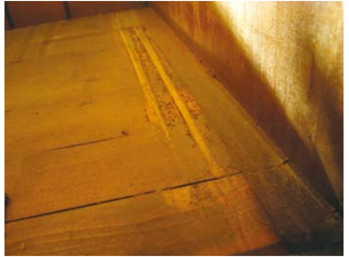
12 Grooves worn in dust boards by drawer runners
