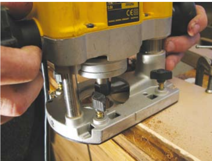
15 Cutting bottom of drawer sides with router collar bearing against MDF straightedge
