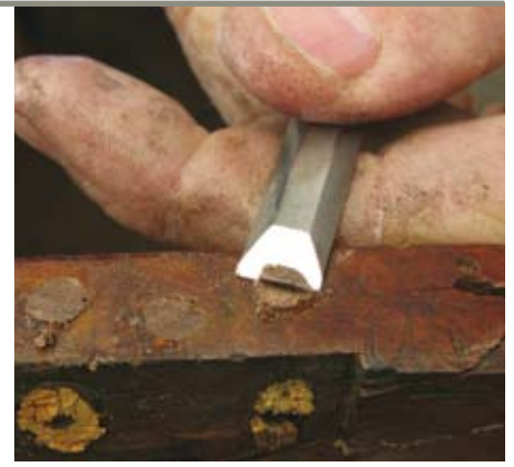
2 Trimming off the dowels inserted to strengthen repair to left of flap
