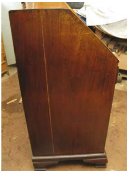
10 Vertical fillet fitted to left-hand side
