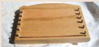
To drill the sides, the end stop should tightly butt up to the back and the side stop against the outside edge. Ensure that the jig is securely held in place, either by clamping or screwing into the end of the piece.
