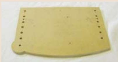
of the cabinet sides, measured from the datum side of the stock. When deciding on the positioning of the front dowels, note that the sides are different widths. Screw a stop to the end of the stock and fix another stop to the datum side.
