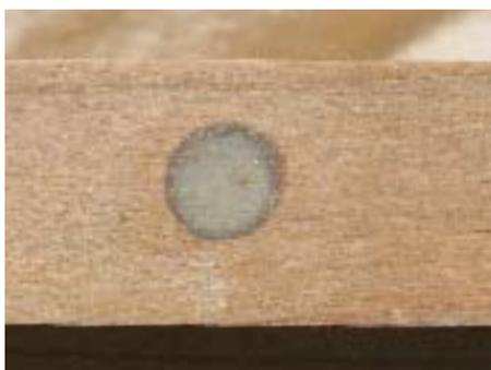
**The magnet fixed in the cabinet side with epoxy, then cleaned up**
