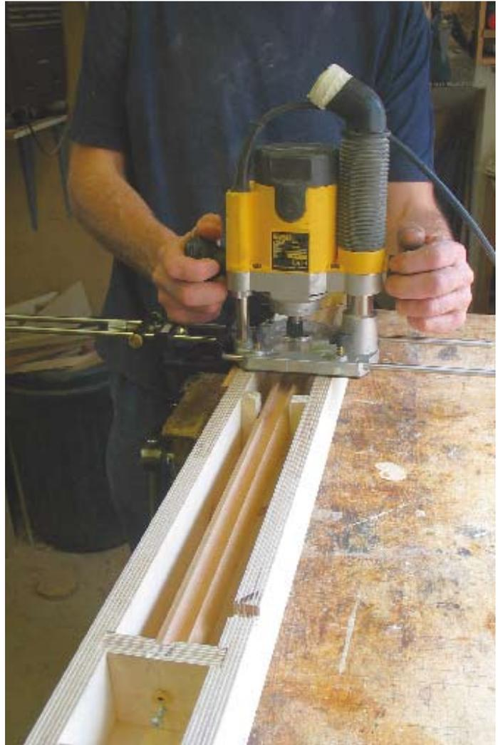
Routing the door column in the jig
