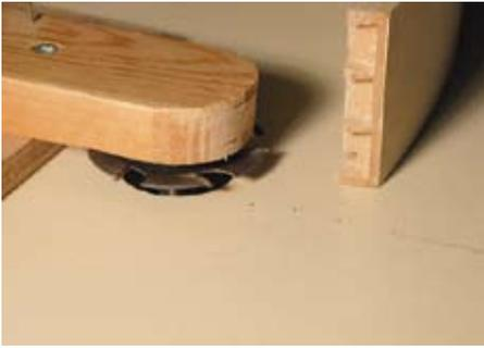
**Make-shift ring fence on router table for cutting grooves in the drawer front (guard removed for photo only)**
