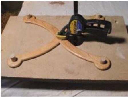
Clamping rails using the jig for positioning
