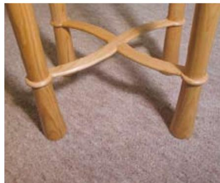
Leg bottoms and rails fitted to mid-sections
