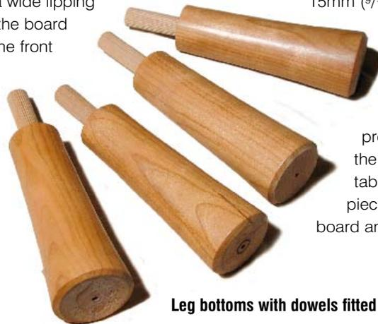
Leg bottoms with dowels fitted
