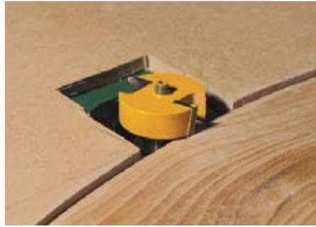
**Rebate cutter and curved fence used to rebate the front of the drawer bottom (guard removed for photo only)**
