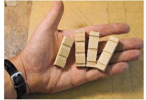
**Cut packing pieces to the exact profile of the drawer and moulding in order to prevent bruising when clamping**
