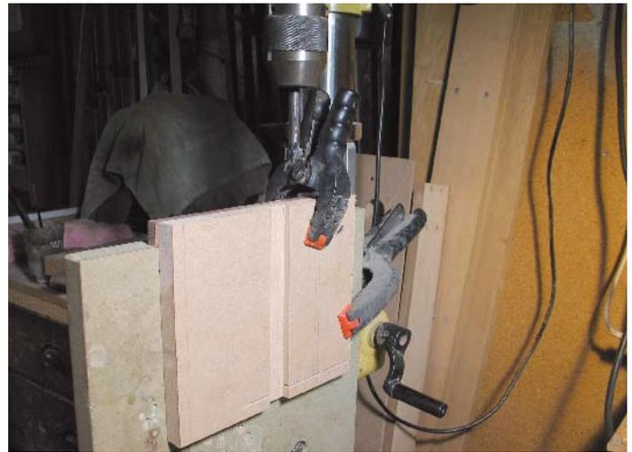
Jig for drilling the leg
