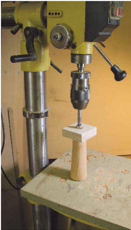
Drilling the foot to receive a dowel
