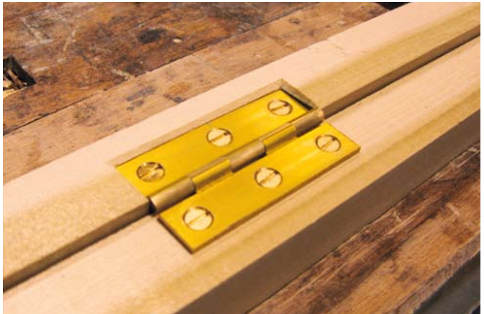
▲ Pic.1 A traditional method is to recess the hinge entirely into the door stile, but the recess has to be chamfered to avoid binding and it has to rely entirely on the screws for support
