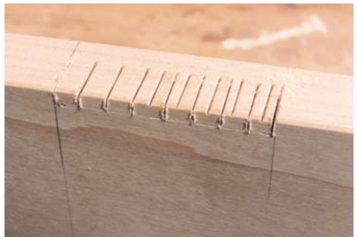
▲ Pic.8 Break up the waste with a sharp chisel and then pare away
