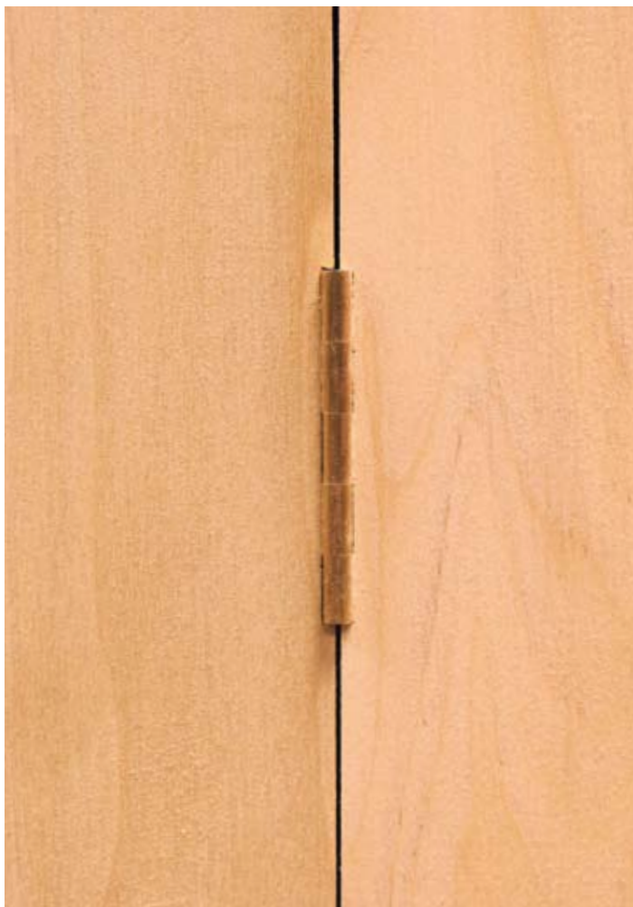
▲ Pic.2 Another traditional method is to set the hinge's leaves equally into both stile and frame. Surely there's a 'third way'? Read on...
