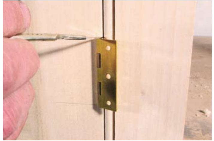
▲ Pic.12 Use a scalpel or marking knife to mark the hinge positions on the edge of frame
