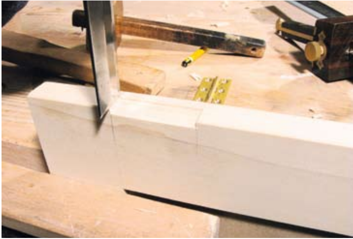
▲ Pic.11 The last task is to locate the chisel in the knife lines and remove the sliver left by the saw
