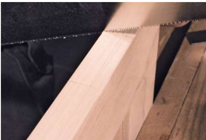
▲ Pic.7 Make a series of cuts into the waste using a saw, sawing slightly shy of the knife lines
