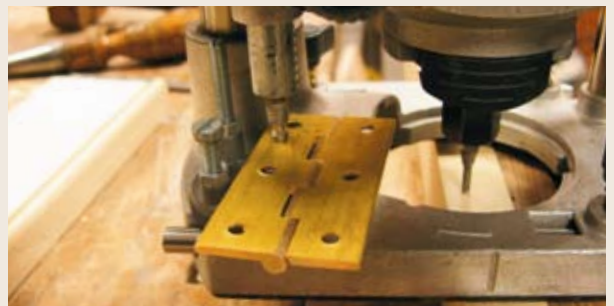
▲ Pic.20 Set the depth to the thickness of the flap by inserting the flap into the depth stop
