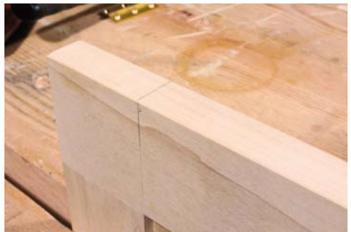
▲ Pic.4 ...then, again lightly, square the pencil lines across the door edge and face
