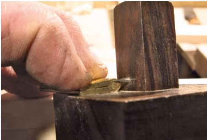
▲ Pic.5 Setting a marking gauge to the width of the hinge to the centre of the hinge pin, gauge between the pencil lines
