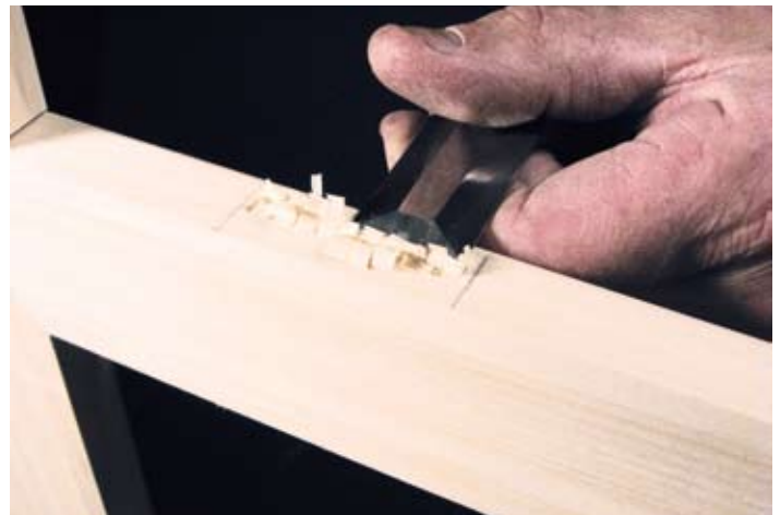
▲ Pic.16 Pare at an angle, stopping just short of the gauge line to create the sloping from front to back
