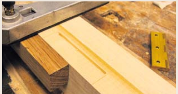
▲ Pic.21 Rout out a groove at the back of the recess, leaving a good clean line
