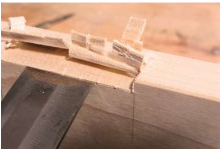
▲ Pic.9 With paring out the recess, creeping up on the bottom gauge line is the best approach
