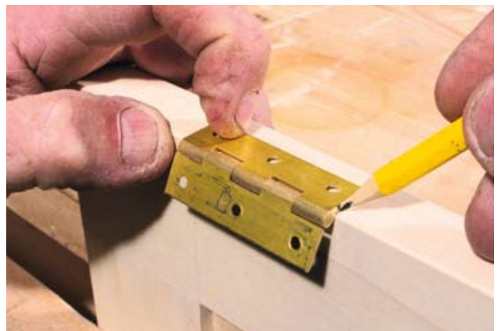
▲ Pic.3 Place the hinges in position and lightly mark out using a pencil...
