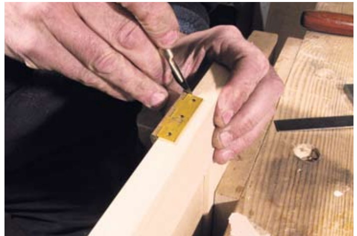
▲ Pic.6 Repositioning the hinge, prick with a scalpel or marking knife then mark around
