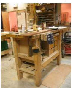
carving or marquetry work the bench could be a couple of inches higher. When making a bench it's probably best to err on the high side, you can always cut it shorter.
