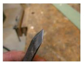
Marking knife. A lot of marking out is done with a knife or scalpel. Marking knives are sharpened on one side, leaving a flat side to go against the square or straight edge. The Japanese marking knives shown are good.
