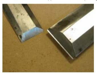
Single bevel. The edge is both ground and honed to a single bevel of 25°, as shown on the chisel on the left. For the beginner buying new tools this system would mean they could get started without having to buy a grinder, simply honing to the same angle that the edge was ground to. You would need to buy a grinder once the edge was damaged. With this system honing will tends to take
