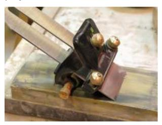
So, for the beginner I would suggest the single bevel system using abrasive on glass and a honing guide. But you will eventually have to get a grinder, then it would be worth switching to the double bevel.
