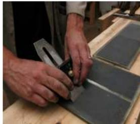
For the beginner I would recommend abrasive on glass, it's cheap and does not require regular flattening. The abrasive could be just wet and dry abrasive stuck to a piece of 10mm glass. Use 240, 600 and 1200 grit and fix them to the glass using Craft Mount spray adhesive. 3M also make some self-adhesive lapping film which gives a nicely polished edge; use 30, 15 and 5 micron grits. But make sure you only press down on the back stroke, else you will dig in.
