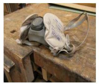
Even with the most efficient extraction there will still be times when a dust mask is useful e.g. Hand sanding. I find the larger moulded masks rather uncomfortable and difficult to seal round the nose, I would recommend a good quality light weight mask with a moulding facility and replaceable filters such as the 3M 2125.
